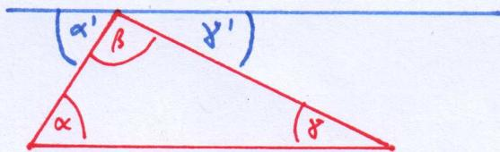
Wechselwinkel  $\alpha' = \alpha$ ,  $\gamma' = \gamma$
